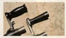
New (left) and old (right) carrying handles with different types of barrel nut latch releases.
